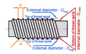
p = pitch of thread  $\alpha$  (alpha) = angle of thread
