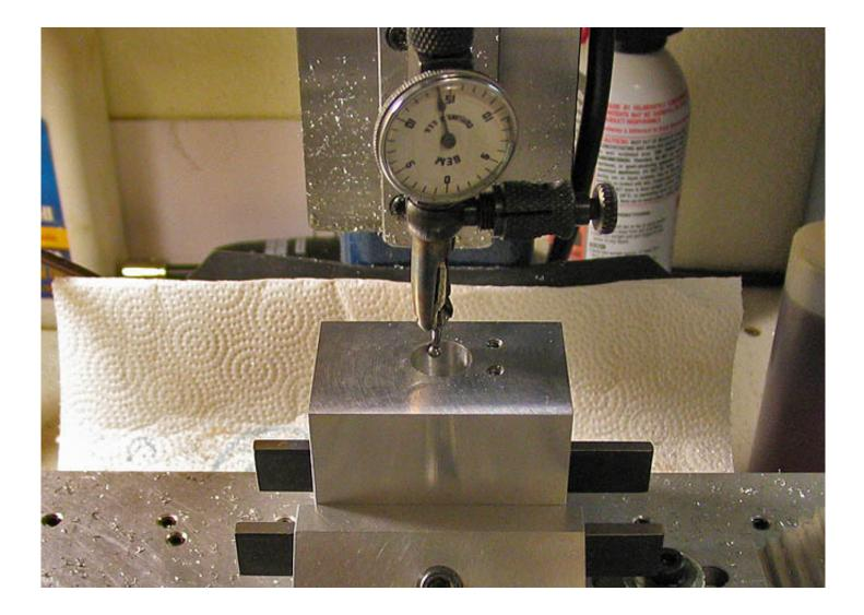
I started by taking the little dividing head to bits, putting the spindle block in the mill, and getting the spindle bore dialed in.
