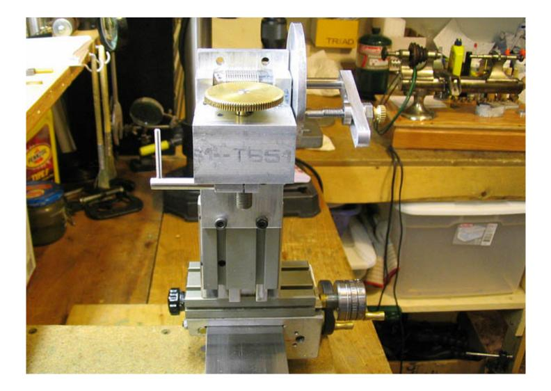
A plate is attached to the back side of the indexer, as seen in this shot, with six mounting holes matching the Taig slide. Only four of the six hole are used at one time, depending on how high the divider needs to sit on the milling column.
