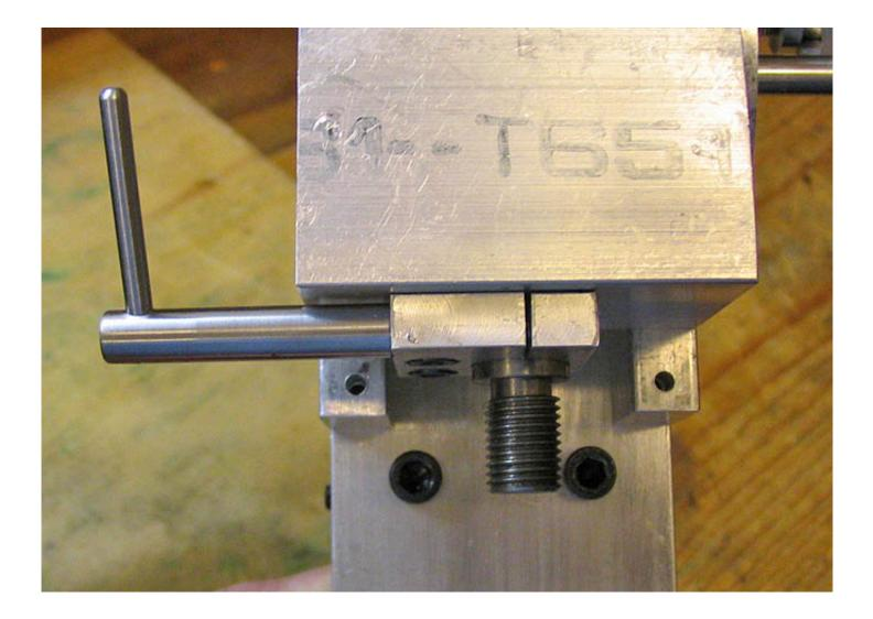
Here you can see how the completed brake assembly fits to the main body.
