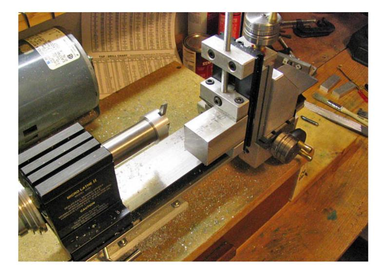
Squaring up the ends of the main body with a fly cutter.
