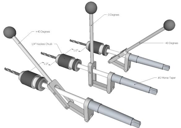
*Pecking* can be a long arduous process. Recently, I drilled a 4-inch deep D-size (0.246-inch D) hole from my lathe's tailstock ram. Eventually, each peck advanced just 1/10-inch. As my lathe's ram travel is short of 4 inches, I eventually had to unlock the tailstock's hold down and slide it back to clear the chips after each peck. Once again I promised to build a Quick In&Out Drilling Actuator for my lathe. This time, however, I turned promise into product.
