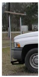
wire feed welder. Rubber pieces were glued to the contact points on the truck to prevent damage to the paint. The bottom pieces of the front support are  $\frac{1}{2}$  by 1- $\frac{1}{2}$  inch channel, while the bed section is 1x2-inch rectangular tubing.
