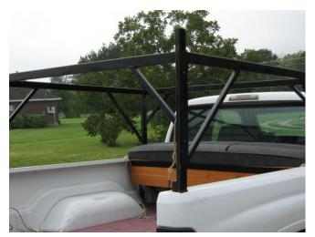
I fabricated an overhead rack for my 1998 Dodge ¾-ton truck. It consists of two sections: the rear bed mounted frame and a front support for carrying long material like pipes and the tubing used to built this project.
