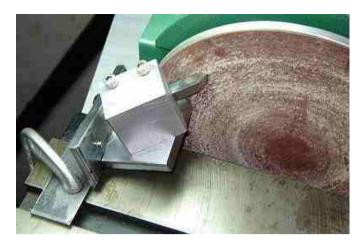
of the wheel is used. When using the left side of the wheel it may be helpful to rotate the toolholder so its slot is on the right side. Alternatively, change only the relief angle and flip the bit itself over to use the same side of the wheel. Lots of ways to use it once you have the jig in hand.
