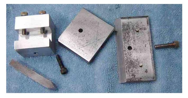
The backplate is HRS 2.5 to 3.5 wide, 1.5 high and 1/4 thick. I used 10-32 socket head fasteners throughout, Cleeve used 1/4". A clearance hole is needed in the backplate 9/16" from the bottom and centered. The bottom edge is beveled (about 45 degrees, leave 1/32 or so on the back edge untouched) on the front to allow tilting the jig about the rear edge in use. The pins are added later to facilitate setting the 10 degree relief angle.
