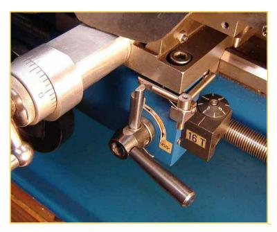
I looked for a minilathe mechanical auto-stop but didn't find one that triggered so the stop point would be reasonably repeatable. Repeatability is needed when the auto-stop will be used for threading, my main use for it. Of course it is also useful for finish passes using fine feed to avoid a crash should you be distracted. This auto-stop works only for imperial threads while the more complex <u>dog</u> <u>clutch</u> auto-stop provides automatic thread pickup for imperial and metric threads.
