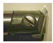
The bit was extended from the bar while sharpening to increase clearance. This picture shows the result, with the bit set for threading. Note how the insert is held at an angle; this angle is what prevented me from using this bar for threading prior to building Cleeve's jig. This bar uses the small HSS inserts, only 100 thou wide.
