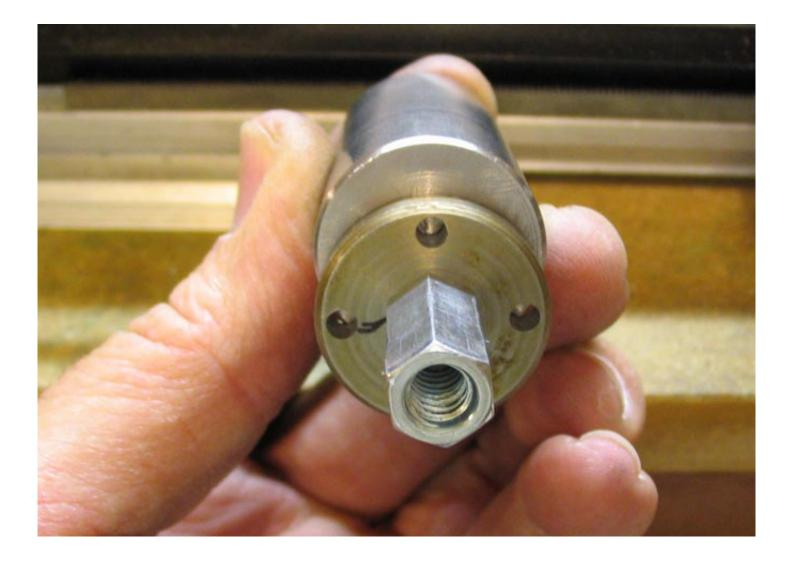
Drill and tap a 1/4-20 hole .250 off center in the end of an arbor that will fit your lathe.
