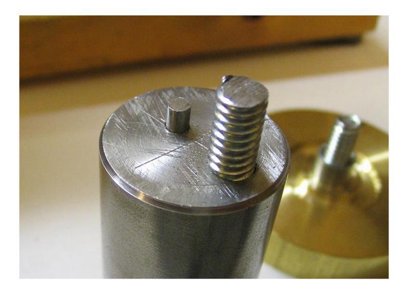
A 1/8" piece of drill rod is now put in the hole with Locktite. The drill rod stud needs to stick up above the surface just under 1/8".
