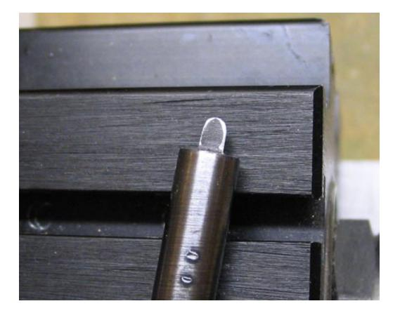
Once ground to the proper shape, the bit is heated to bright red heat and
