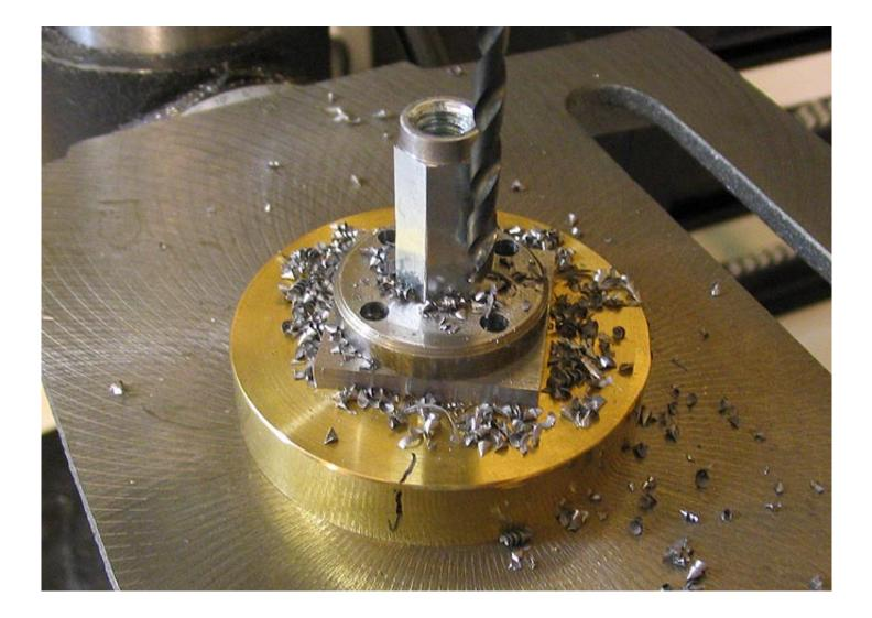
Place the drilling template over the piece of tool steel, which will become your cutter blank,
