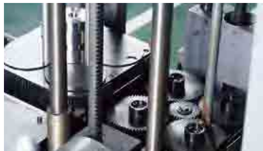
SRO Round Rack used as a work storage device (fluctuating table) of the auto loader.
