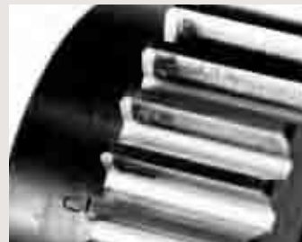
Poor tooth contact and pitting
