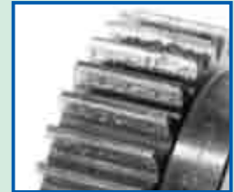
Example of defacement due to insufficient surface durability.
