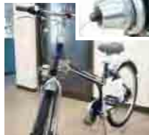
2WD Bicycle by SHESCO SB Bevel Gears are used in the driving components in both the front and rear wheels.
