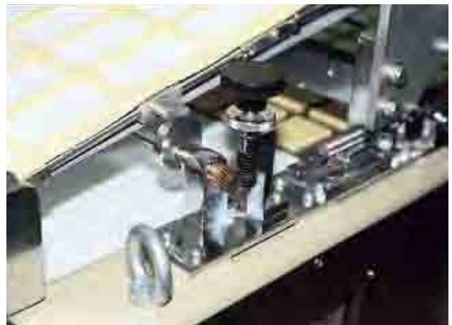
SW Worms and BG Worm Wheels used in adjusting a cloth feeding device
